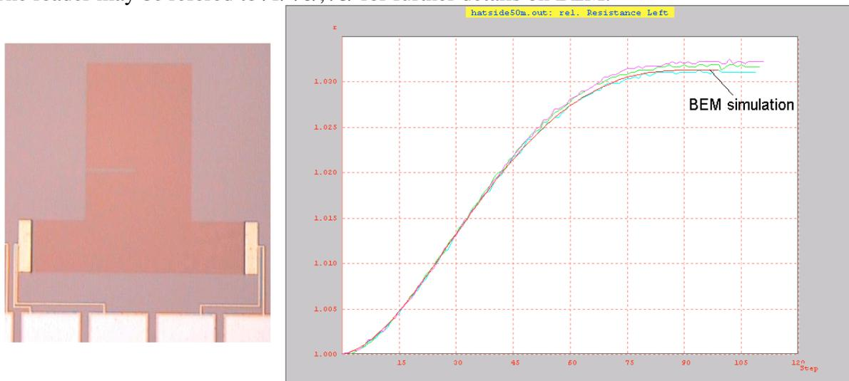
**Fig. 2** Three measured trim characteristics of the same top-hat side-cut in comparison to the numerical result
