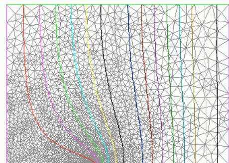
**Fig. 1** FEM solution of a 3-side bar resistor
