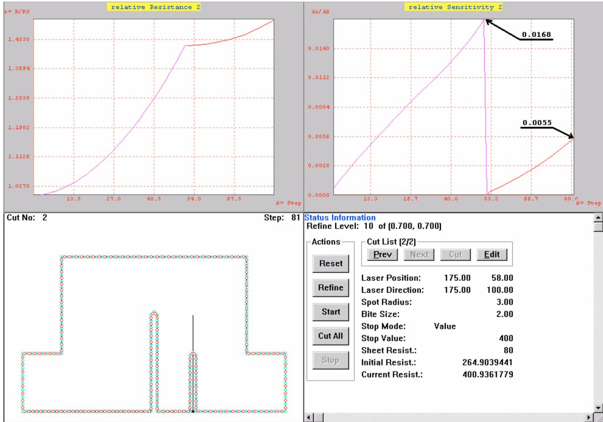
Fig. 4 Simulation result of the double P-cut for  $R_S - \Delta R_S = 80 \Omega/sq$
