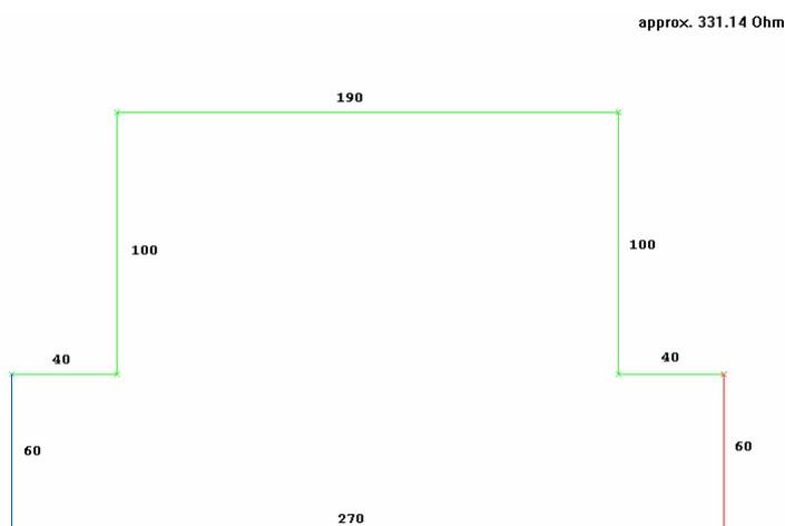
**Fig. 3** Resistor shape candidate with approx. 331  $\Omega$
