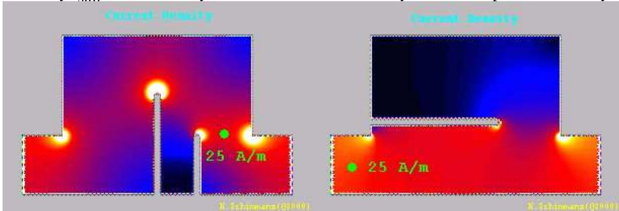
**Fig. 5** Current density maps of maximum trim lengths and used sample points (left:  $80\Omega/sq$ ; right:  $100\Omega/sq$ )
