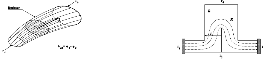
Fig. 1. Left : General Resistor; Right : Top-Hat film resistor with highly conducting terminals \Gamma_1 and \Gamma_3 and laser cut at \Gamma_2 (called plunge- or P-cut)
